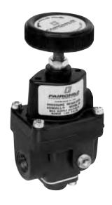
The Model 30 is designed for applications that require high capacity and accurate process control in a small package. A poppet valve which is balanced by utilizing a convoluted diaphragm, insures a constant output pressure even during wide supply pressure variations. Stability of regulated pressure is maintained under varying flow conditions through the use of an aspirator tube which adjusts the air supply in accordance with the flow velocity.
